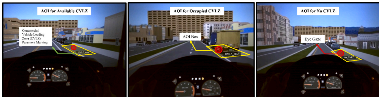
Fig. 2. Example of a truck driver fixation pattern on pavement marking area of interest (AOI) and how AOIs were drawn and identified.
