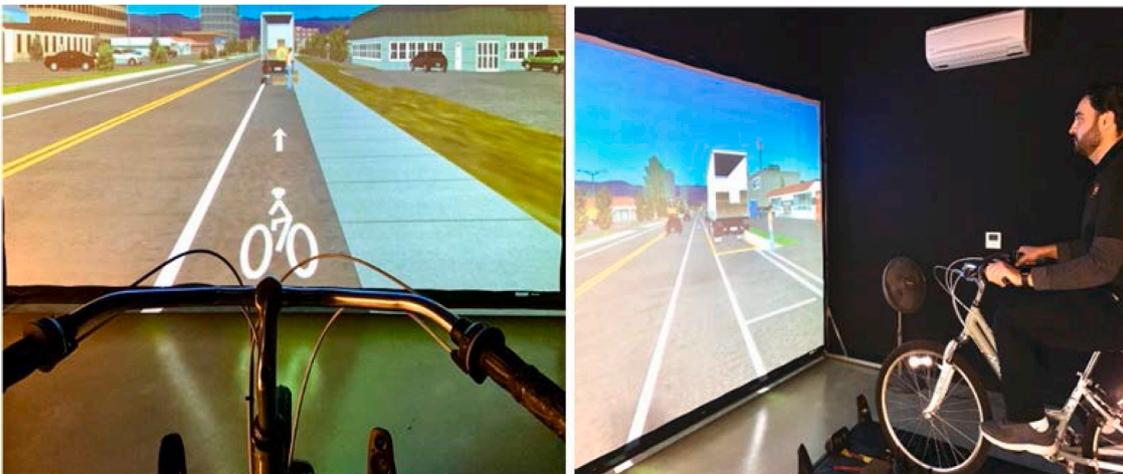
Fig. 1. Simulated environment in the OSU bicycle simulator; Participant's perspective (Left); Researcher testing the environment (Right).
