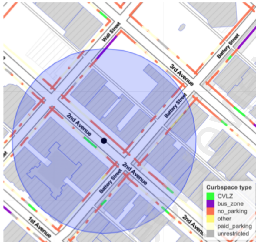
Figure 2 – Curb parking allocations to different vehicle types contained in a 100-meter diameter buffer centered at a delivery destination were considered as predictors in the cruising time prediction model
