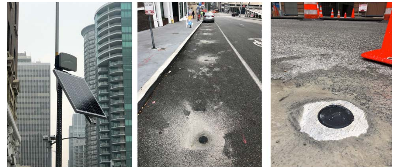
Figure I.1.1 The left picture shows one of the gateways installed in Belltown, Seattle, which collects sensors' data and sends it to the cloud; the center picture shows a passenger load zone with sensors installed; right picture shows a close-up photo of one sensor.
