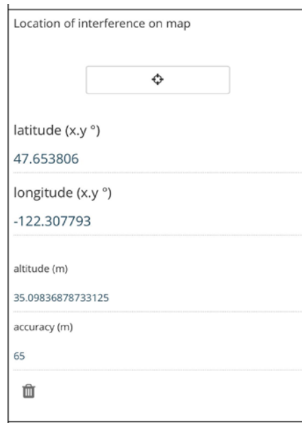
Figure 62: Location example: once you press the “Find my location” button (shaped like a target) it automatically loads the latitude, longitude, altitude, and location accuracy.
