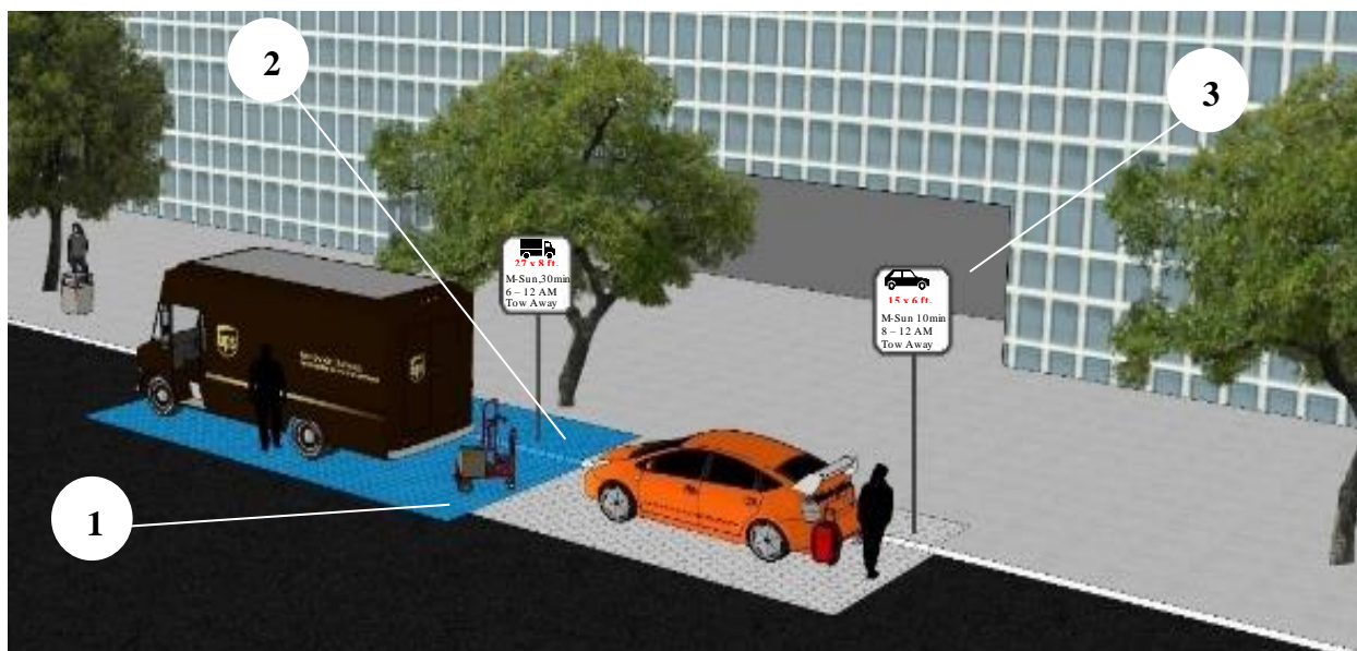
Figure 15 Rendering of Curb Space Redesigned for 27x8 ft. and 15x6 ft. vehicles (Toyota, 2018) UPS Truck Dimensions courtesy of Anna Alligood and Siqi Lu
