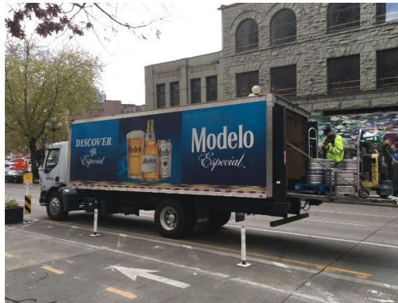
Figure 18 Lift Gate Engaged (Sheth, 2017-2018)
