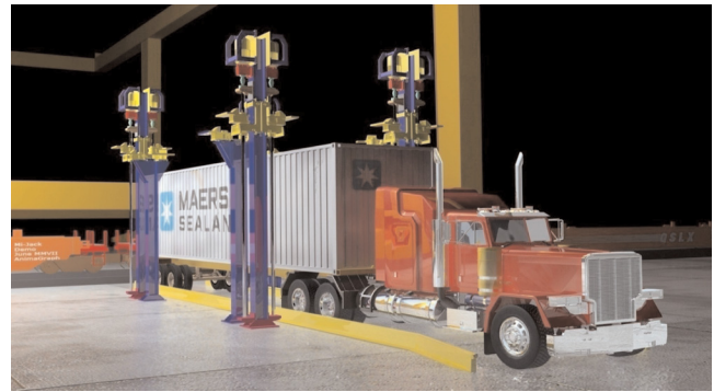
FIGURE 2 Two-high ATMS positioned under WSG crane and perpendicular to loading tracks.
