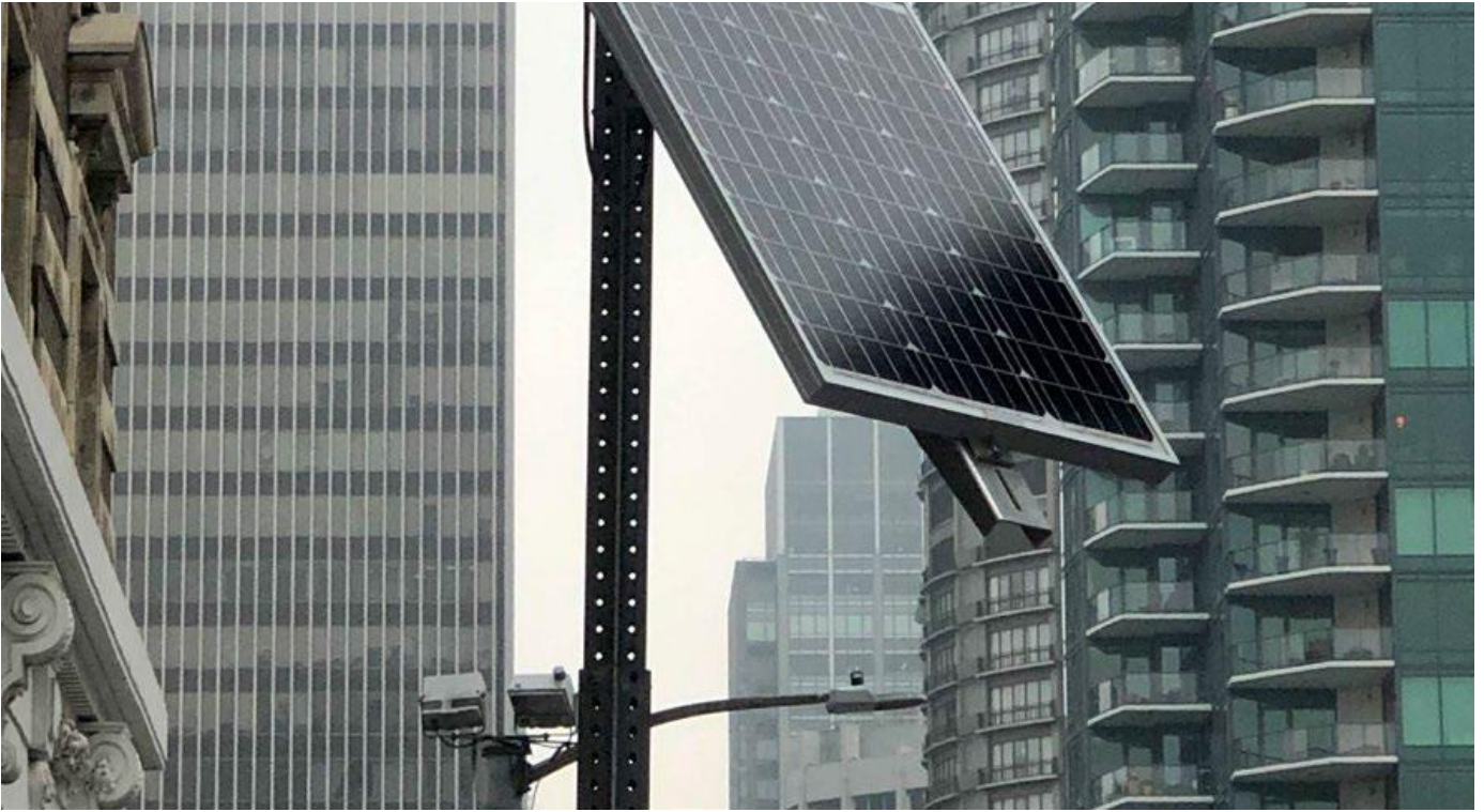
Figure 4: Deployment of curb availability sensors on a passenger load zone and commercial vehicle load zone in Seattle, WA274 curb parking availability sensors were installed on commercial vehicle load zones and passenger load zones
