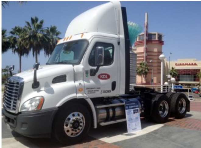
Figure 10. Liquefied natural gas large Class 8 truck used in grocery store pilot program (fleetsandfuels.com)
