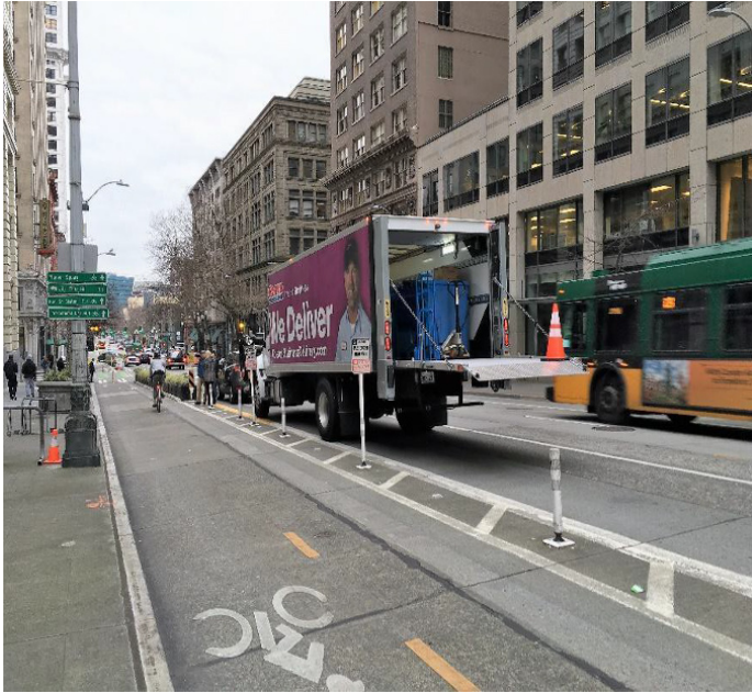
Figure 21.1. Second Ave. sidewalk, bike lane, CVLZ, through lanes, and bus stop in downtown Seattle. For a color version of this figure, see www.iste.co.uk/taniguchi/cities2.zip
