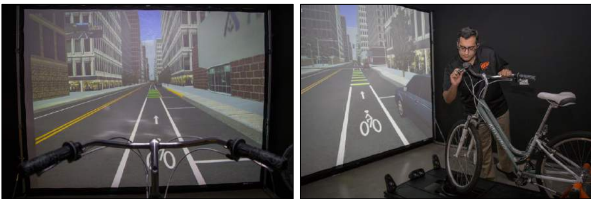
Figure 3.3 Simulated environment in the OSU driving simulator. Left: Participant's perspective. Right: A researcher checking a bicycle brake.
