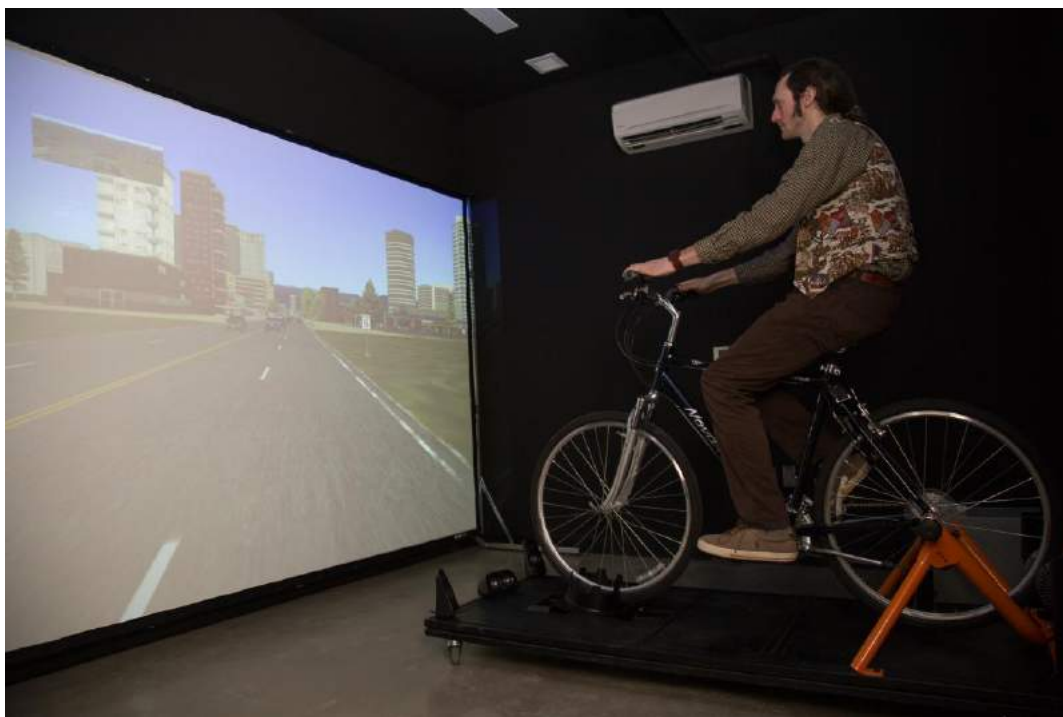
Figure 2.10 Bicycle simulator at Oregon State University (OSU)
